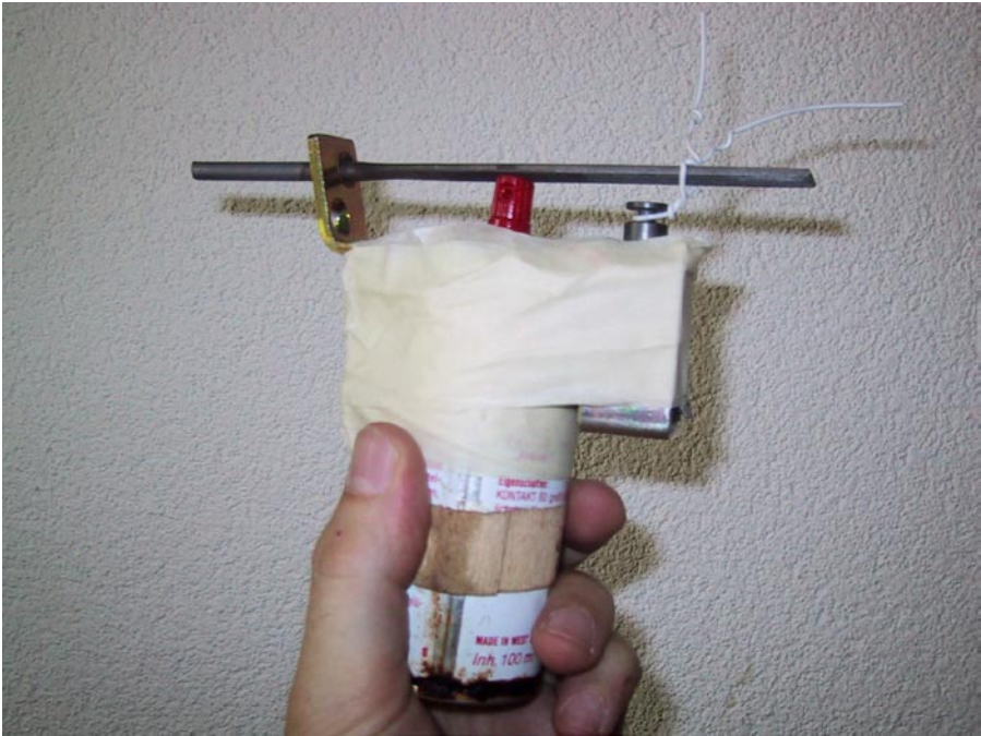
CAN-HOLDER : A first prototype for the spray-activation mechanism. An electromagnet with a movable iron core is used to pull the lever that pushes on the nozzle.
