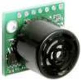
**Getting started with the Maxbotix sonar sensor - quick start guide** by adafruit
