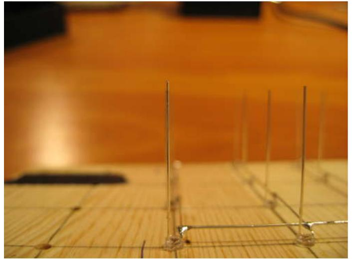
**Step 24: Build the cube: bend the pins**
