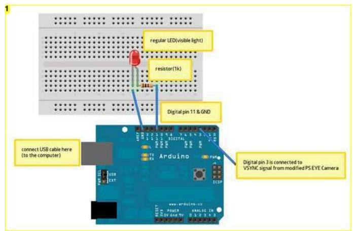
1. Before soldering the 30 gauge wire to V-Sync, a test should be performed to ensure all connections are correct. Build the circuit below. When the 30 gauge wire contacts the V-Sync via, the LED on the breadboard should flicker rapidly.
