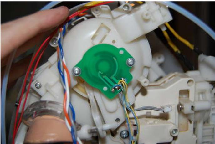
**Step 15: Getting the morors and sensors connected to the arduino.**
