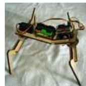
**simpleWalker: 4-legged 2-servo walking robot** by edwindertien
