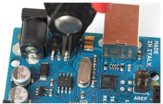
Then you'll need to heat the tab up to get it liquid so you can lift off the old part. Although it may seem counter intuitive, its best to **add** some solder to the tab, melt it on with your iron, this will improve the heat conduction since the tab is so large.
