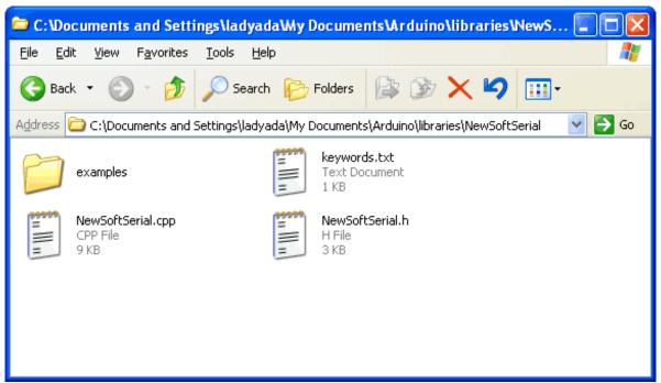
There may also be some **.o** files. The **.o** files are C++ compiled Objects. If you end up working on the library and modifying it, be sure to delete the **.o** files as that will force the Arduino IDE to recompile the modified **.cpp**'s into fresh **.o**'s.
