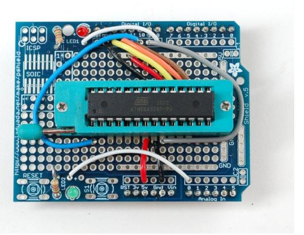
With the USB cable still plugged in (and the same Serial port selected as before) Select Tools→Burn Bootloader→w/Arduino as ISP
