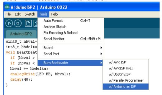
On newer versions of the Arduino IDE, select **Arduino as ISP** from the **Tools Programmer** menu, then select **Burn Bootloader** from the Tools menu.
