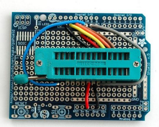
Follow the protoshield tutorial to solder in the Red LED into **LED1** position, Green LED into **LED2** position. Also solder in the two 1.0K resistors next to the LEDs. We'll use the LEDs as indicators. Then solder a wire from the LED2 breakout (white) to analog 0 and a wire from LED1 breakout (white) to digital 8.
