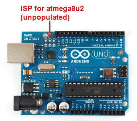
The code for the 8u2 is based on LUFA, Dean Cameran's totally awesome USB-AVR library that has great examples and documentation. Its also completely open source. Does the Uno use a resonator or a crystal for the processor clock? The FT232RL had an internal oscillator whereas the 8u2 does not. That means there is a 16mhz crystal next to the 8u2 to allow it to keep up with precise USB timing.
