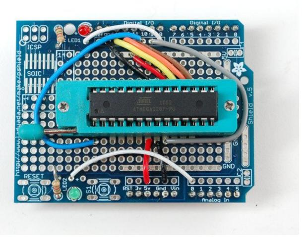
Finally, you'll need to solder on the header to allow the shield to be placed on, break the 0.1" male header and place it into the Arduino sockets. Then place the shield above on top to solder it in place.
