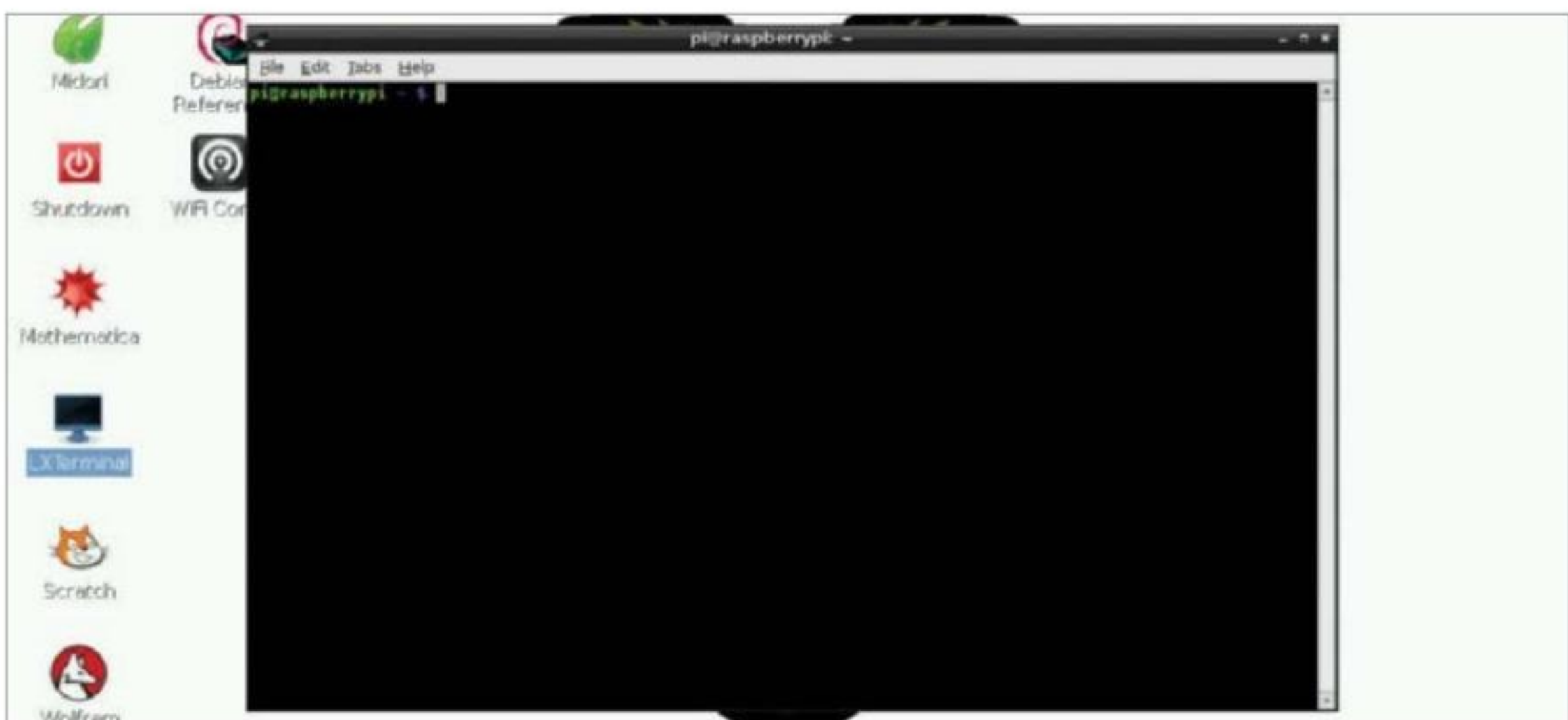
Fig 1: The terminal emulator allows you to access the command line while still being in the desktop environment
