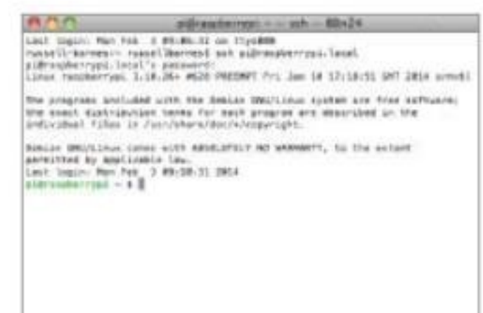
Fig 2: The Avahi tool enables you to log into your Pi via SSH by name, rather than needing to discover its IP address
