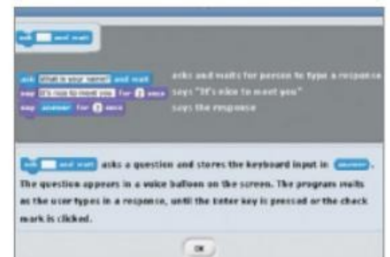
Fig 4: Block Help Window – Example of the help window associated with an 'ask and wait' block
