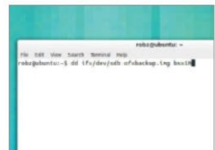
Fig 3: The dd tool is what you'll use on a Linux and Mac computer, and it's available by default in the terminal emulators
